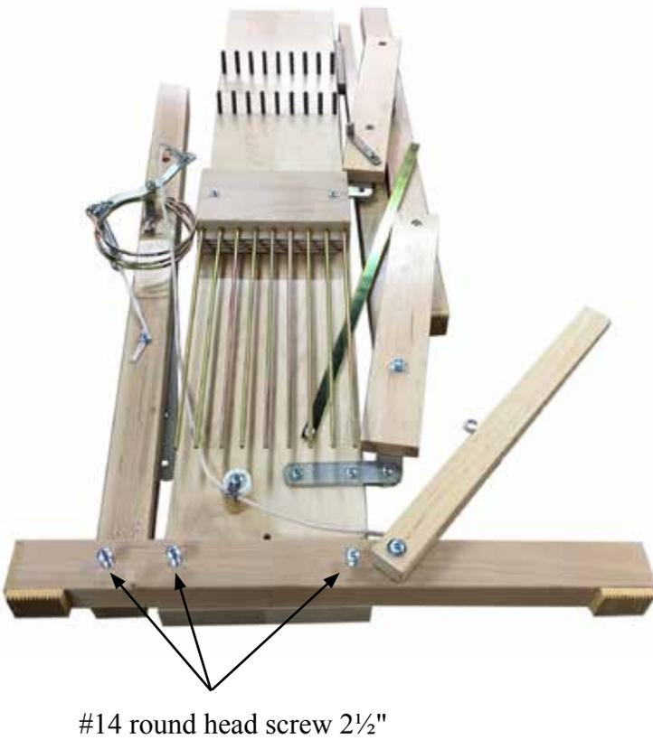
Lay the right side on the floor with caution (you can put a piece of cardboard on the floor). Removed the packing material and using three #14 round head screw 2½", affix the base (the brake treadle is already installed) to the right upright and the back post to the base.
