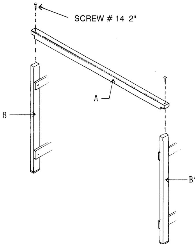
Using two 2" (50 mm) round-headed screws no. 14, affix one of the two breast beams to the top of the front posts B and B`
