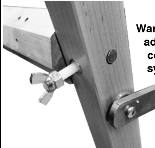
This system will eliminate excessive warp yarn advance when releasing the brake system at cloth take-up. This friction system is adjustable and have to be released when winding the warp on. Just screw the wing nut with nylon bolt to the left back post. Screw in to increase the friction or unscrew it to release.
