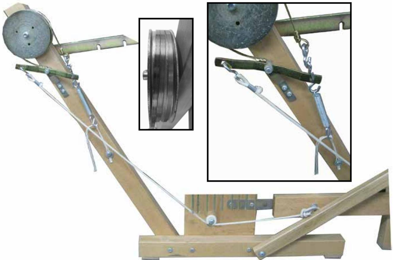
Join the front "S" hook of the brake lever to the brake loop cord so the tension on the spring will be high enough to lock the warp beam while weaving.
