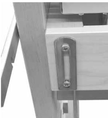
After the Jack box is installed, remove the two screws at the back right corner of the jack box, install the metal protection plate and reinstall the screws to hold it in place. This plate protects the wood from damage by the brake lever when the back beam of the loom is folded in.
