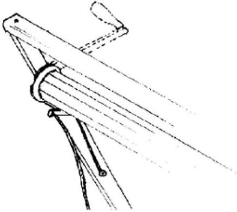
Using two 2" round-headed screws no 14, affix the breast back beam to the back posts.
