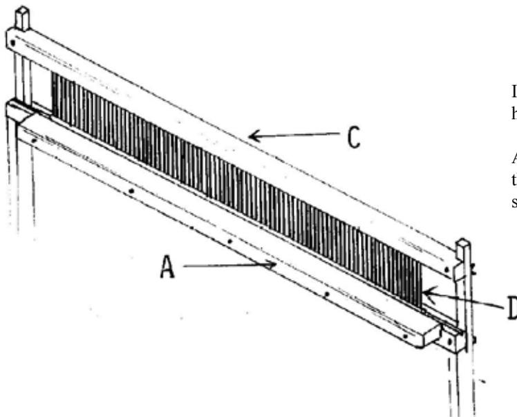
Install reed D in the slots of batten handtree C and batten sley A.
