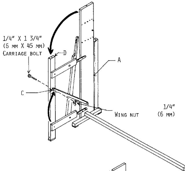
Unfold the front section of left-hand side A. Using a 1/4" x 1 3/4" (6mm x 45mm) carriage bolt and a 1/4" (6mm) wing nut, affix metal hook C to left-hand side front post D.
