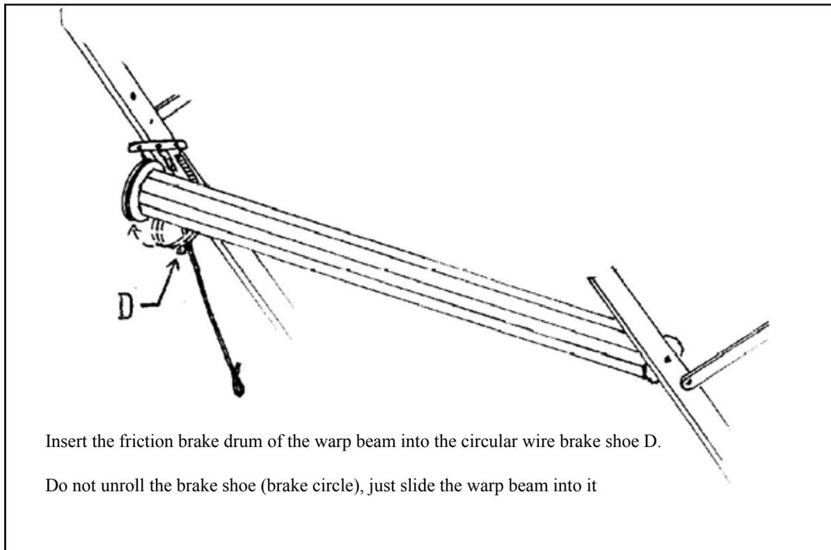
Insert the friction brake drum of the warp beam into the circular wire brake shoe D.
