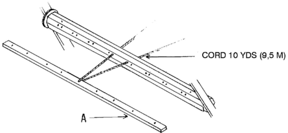
Thread the 10 yard (9 m) cord through the middle hole of beam stick A. Then pass the two ends (equal in length) of this cord through the middle holes of the warp beam.
