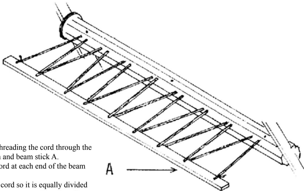
Continue threading the cord through the warp beam and beam stick A. Knot the cord at each end of the beam stick. Adjust the cord so it is equally divided and keeps the beam stick straight. This will reduce warp wastage.
