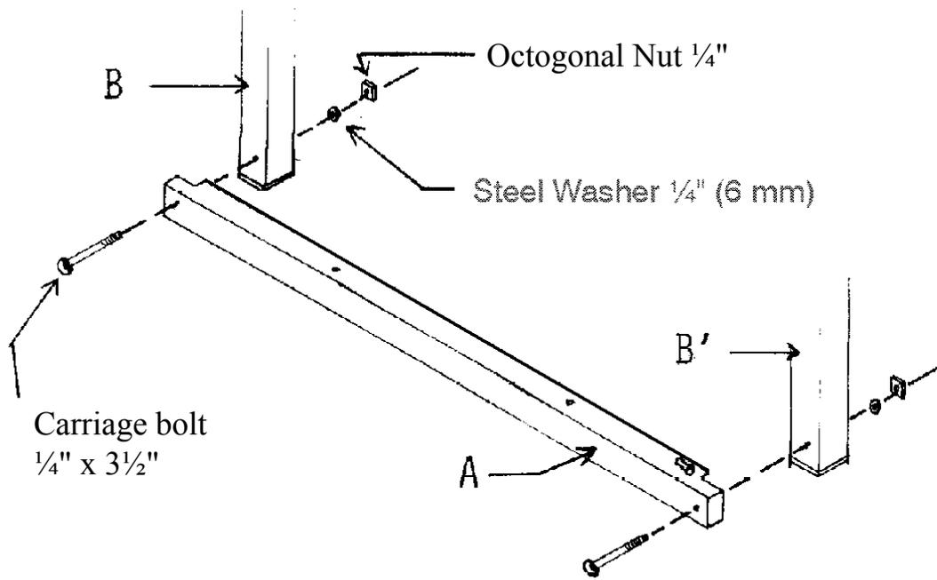
Using two 1/4" x 3 1/2" (6 mm x 89mm) carriage bolts, two 1/4" (6mm) steel washer and two octagonal nuts 1/4", attach the front cross-member A to front posts B right and left.
