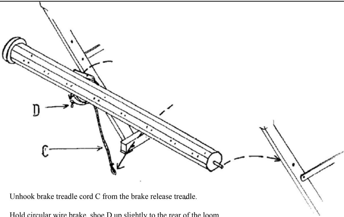
Unhook brake treadle cord C from the brake release treadle.
