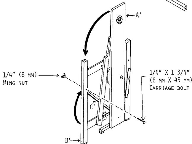
Using a 1/4" x 1 3/4" (6mm x 45mm) carriage bolt and a 1/4" (6mm) wing nut, affix metal hook C' to right-hand side front post D'.
