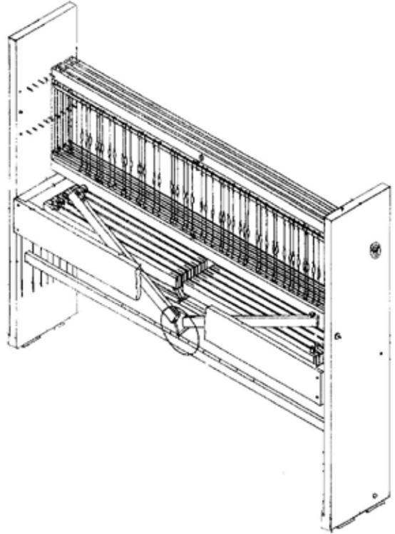
Join the "S" hook of the jacks D to the eyelet of the FLOATING lam E.
