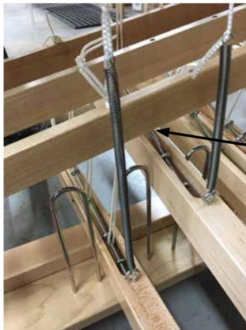
Spring under tension when the treadle is down
