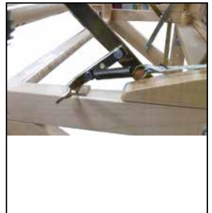
Brake lever closed to tighten the brake cable.
