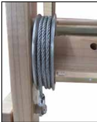
Brake assembly with brake cable. Make sure that it is properly in place.
