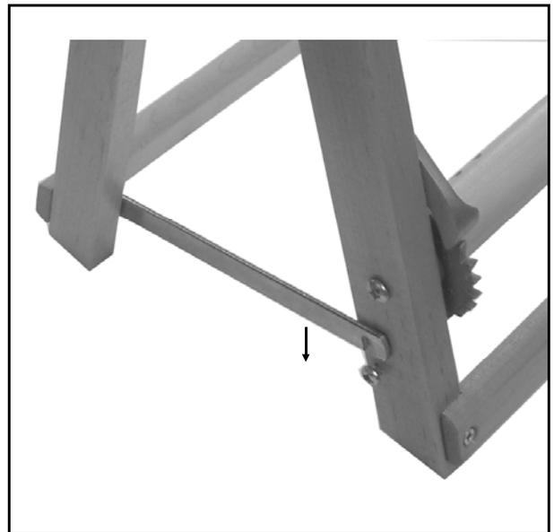
Open the back post assembly and latch the hooks. Set the screws to a snug fit.
