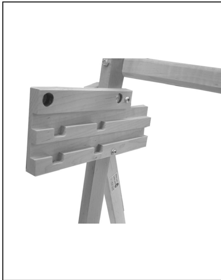
Affix the sliders with the 2 machine screws (M) and 2x 3/16" washers (W) to the metal inserts in the main frame. Then secure using the #12, 1 1/4" screw (S) "
