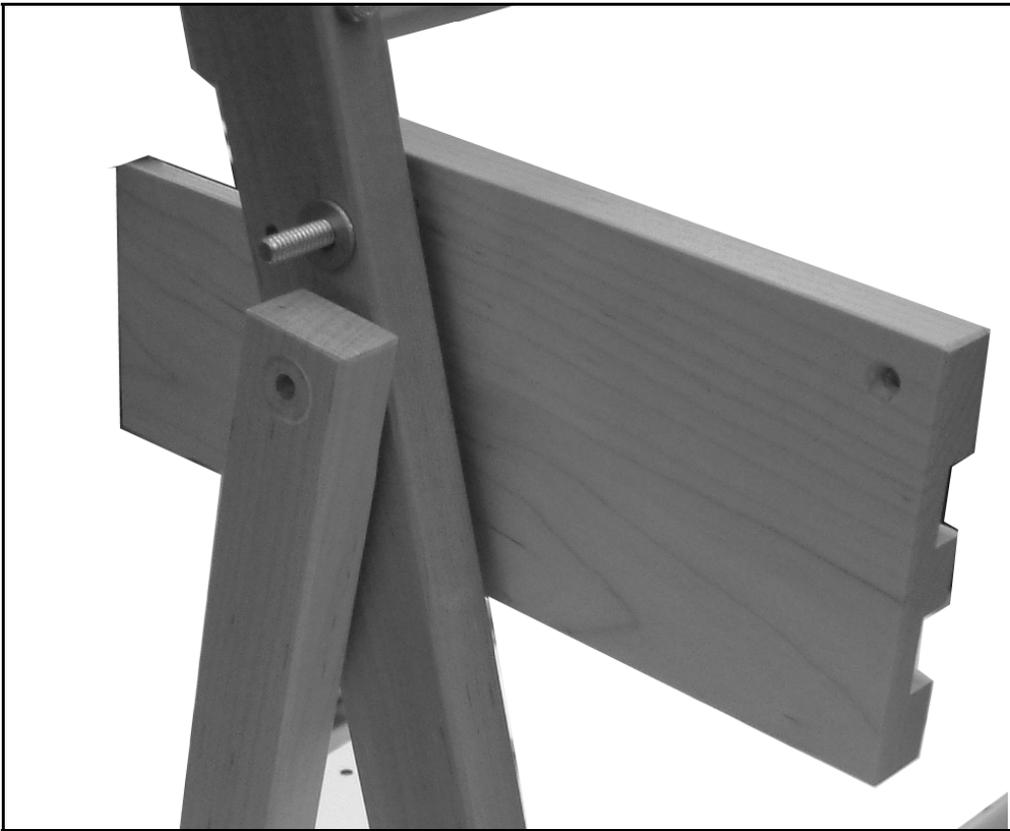
Using the 2.5" x 1/4" carriage bolts, assemble the sliders and the back post assembly to the main frame.
