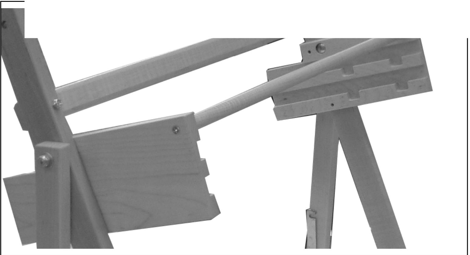
Install the middle slide post using the 2, #8, 1" flat headed screws. Do not overtighten. If the reeds do not slide properly, loosen the slide post slightly.
