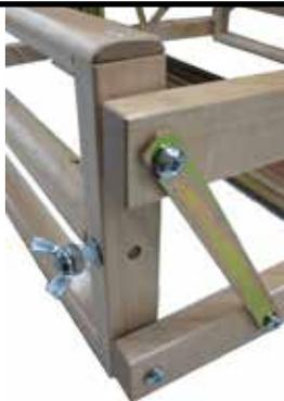
This system will eliminate excessive warp yarn advance when releasing the brake system at cloth take-up. This friction system is adjustable and has to be released when winding the warp on. Just screw the wing nut with nylon bolt to the left back post. Screw in to increase the friction or unscrew it to release.
